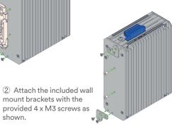
3 Fix the unit to the surface using two appropriate screws (screws not provided)
